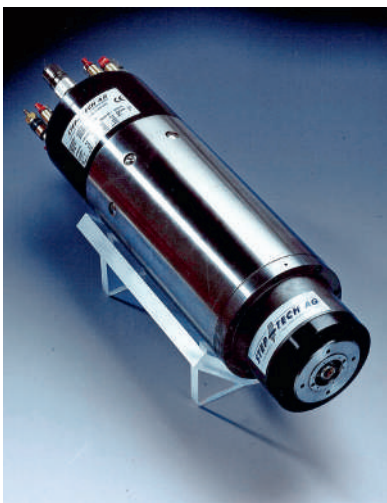
The HVC 140 spindle was the first high-speed spindle manufactured in series by STEP TEC. With a speed of 42,000 rpm on ceramic hybrid bearings and in combination with the 1 g axis acceleration of the HSM 700, it made industrial high-speed milling a reality for the first time in 1996
